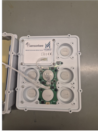
Particle sensor in the lid, cable plugged in
