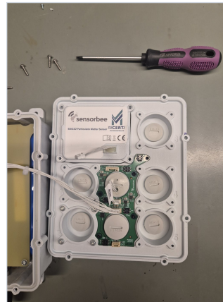
Cable unplugged, screws removed
