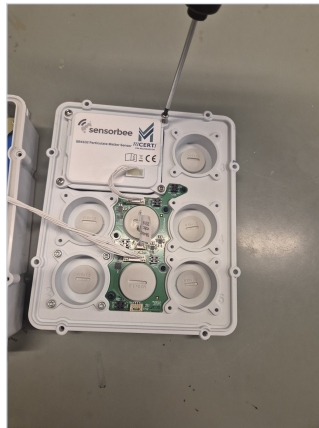
Unscrewing the sensor screws
