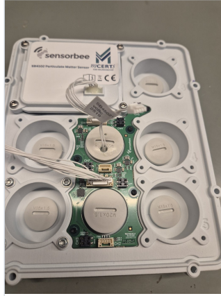
Cable unplugged from the board
