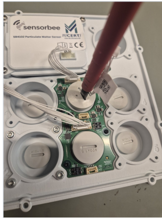
Unscrewing with the flat screwdriver
